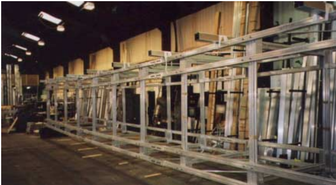
Fig 5: Prototype 15m span gantry prepared for load testing.
