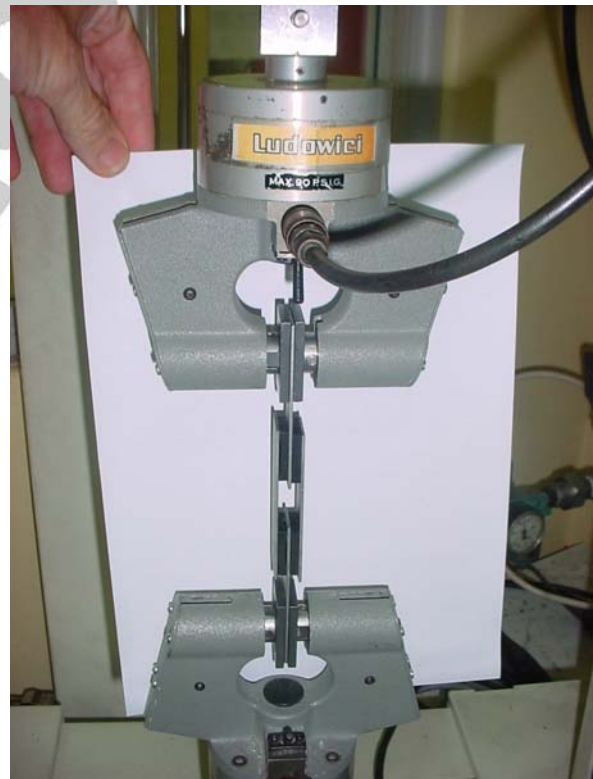
Fig 10. Quad- shear testing to determine the “true” value of the shear modulus, G. Note that the four small rubber samples are bonded to the grip plates for this test, and there is no compression applied. This value is now the basis for designing LE bearings to AS5100.4, having displaced “eb” in these equations.
