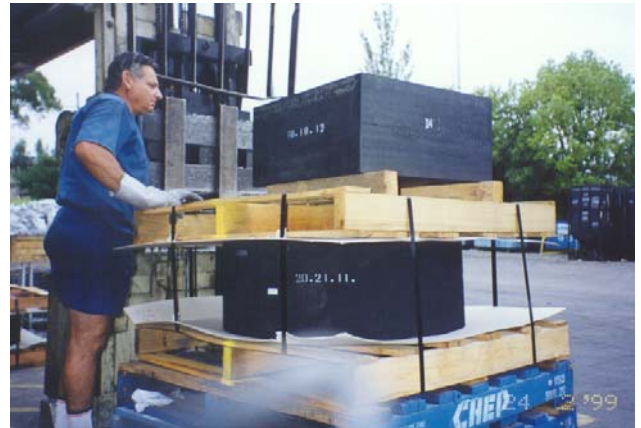
Fig 5a.. Top Left – Melbourne’s Westgate Freeway brgs (up to 750x1050x330) are massive 18 MPa designs. “Ahead of their time”, they were built in the mid 80’s, and include keepers to prevent slip or “walking”.
