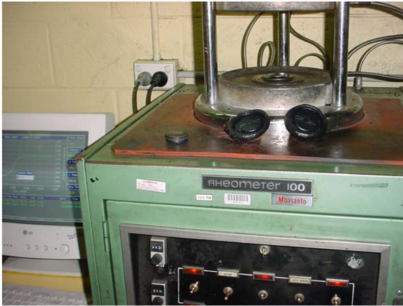
Fig 7a. – Left – Curemeter to check the correct batching of components. Note samples collected before and after test.
