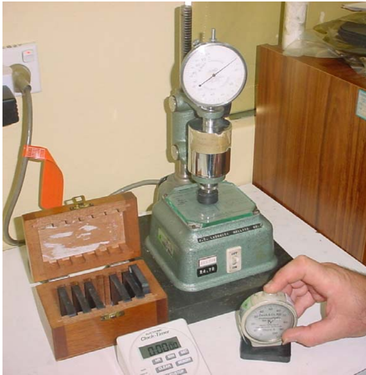
Fig 8a. IRHD Hardness Tester (International Rubber Hardness Degrees) in the background. This is a laboratory machine operated at controlled temperature (23 +/- 2degC), and carefully timed at 30 seconds (method N as specified).
