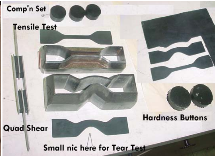
Fig 11a. Top- Samples for testing are moulded and cut from thin sheets. This shows some of the knives and samples for the tension test, the quadshear test, the tear test, compression set and hardness buttons. Most are quarterly tests, although hardness checks are required on EVERY batch, and quad shear is yearly (with low temperature and ozone tests).
