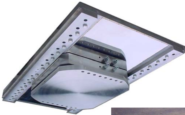
Fig 12b. Bayu Undan Gasfield, Timor Sea. This bearing is of stainless steel, and designed to operate in an aggressive off-shore marine environment at high temperature. Note the polish of the slide counterface, and the (extremely rare) ability to regrease the slide face.
